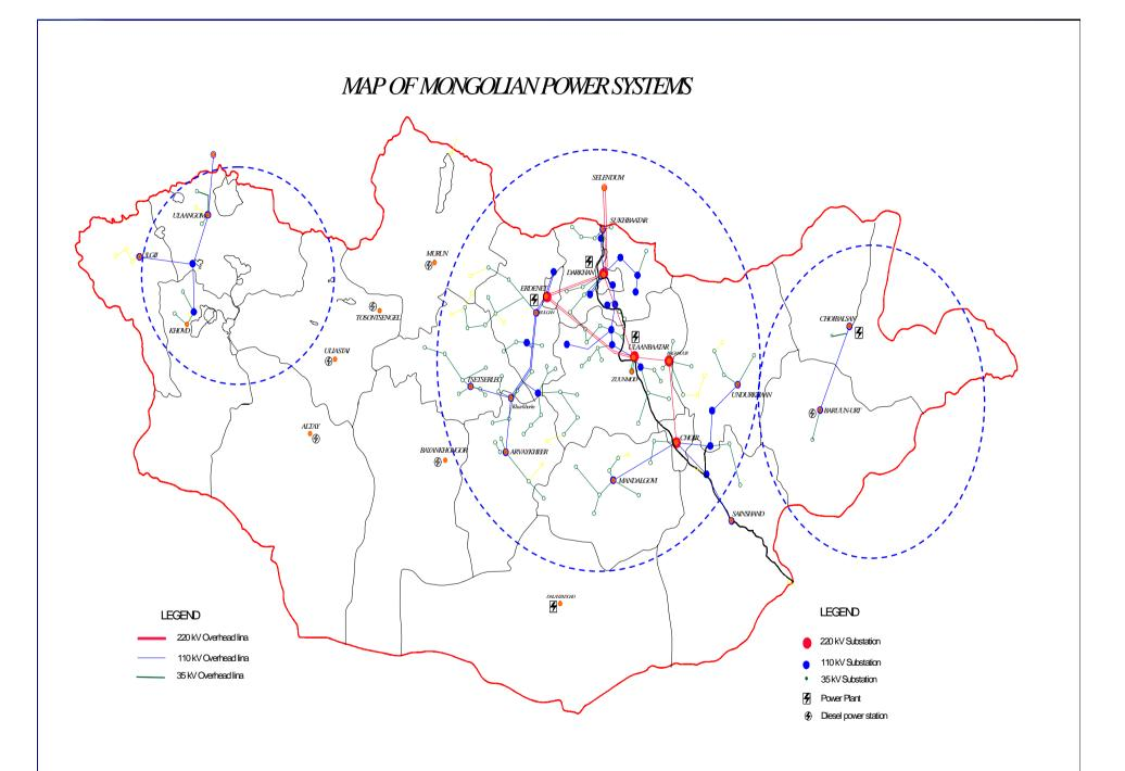
Total installed capacity788.8 MWNumber of power plants5Transmission & distribution companies5Electricity output2.3 GwhTransmission & distribution losses25.0 %Peak load540 MW
