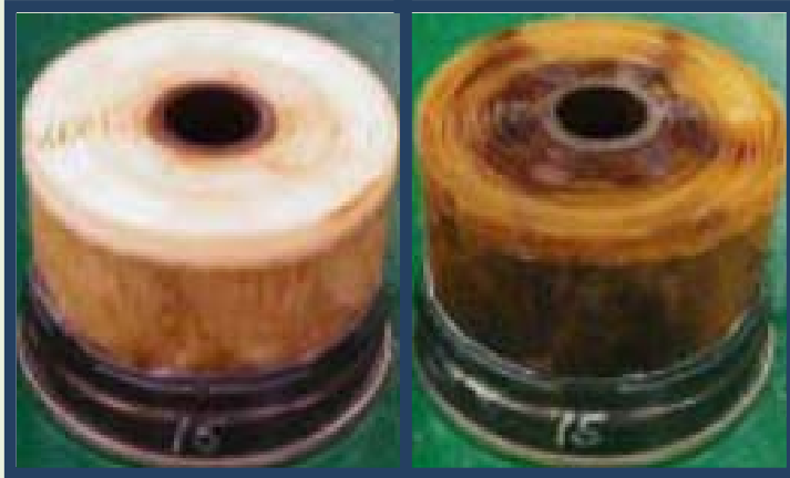
Fuel filter clogging (by impurity)
