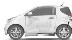
Placement of ultra-thin fuel tank under floor
