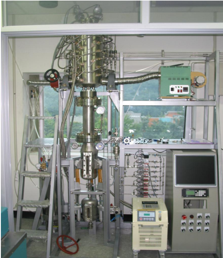
Compact heat-exchanger typed F-T reactor
